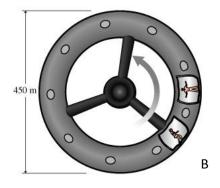
The acceleration needed on the opposite side is in the opposite direction so the forces balance out meaning no resiltant force on the space station as a whole.
